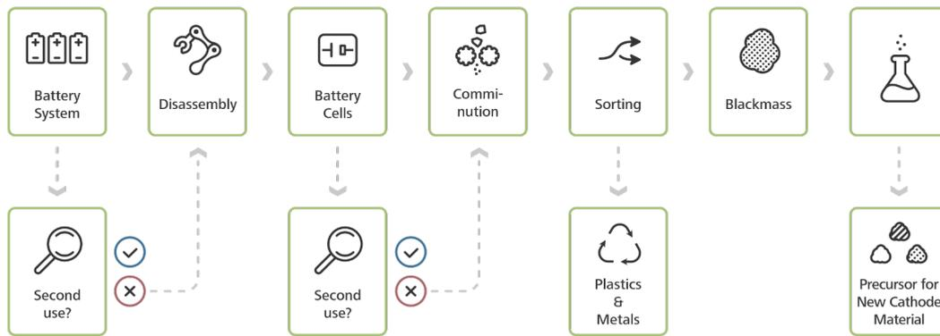
Figure 4.8: Approach of dismantlement and recycling of aged electric vehicle batteries including diagnostics
