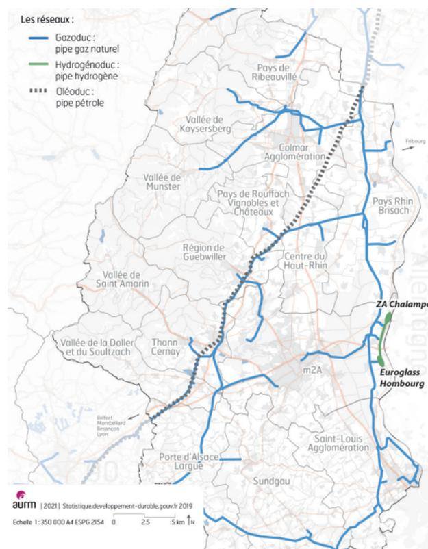
Fig. 5.11: Gas and petrol pipelines in the Mulhouse area (AURM, 2021<sup>6</sup>).
