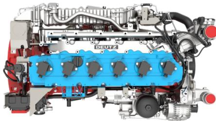
Fig. 5.23: TCG 7.8 H<sub>2</sub> is the first hydrogen engine from DEUTZ ready for the market
