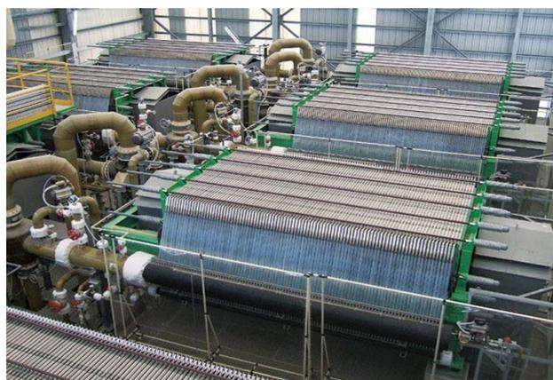
Fig. 5.13: Typical large scale electrolyser set-up (Thyssen-Krupp<sup>7</sup>)
