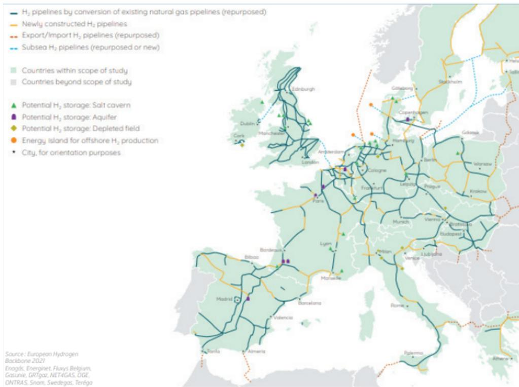
Fig. 5.10: Planned European Hydrogen Backbone<sup>5</sup> (Guidehouse, 2020)
